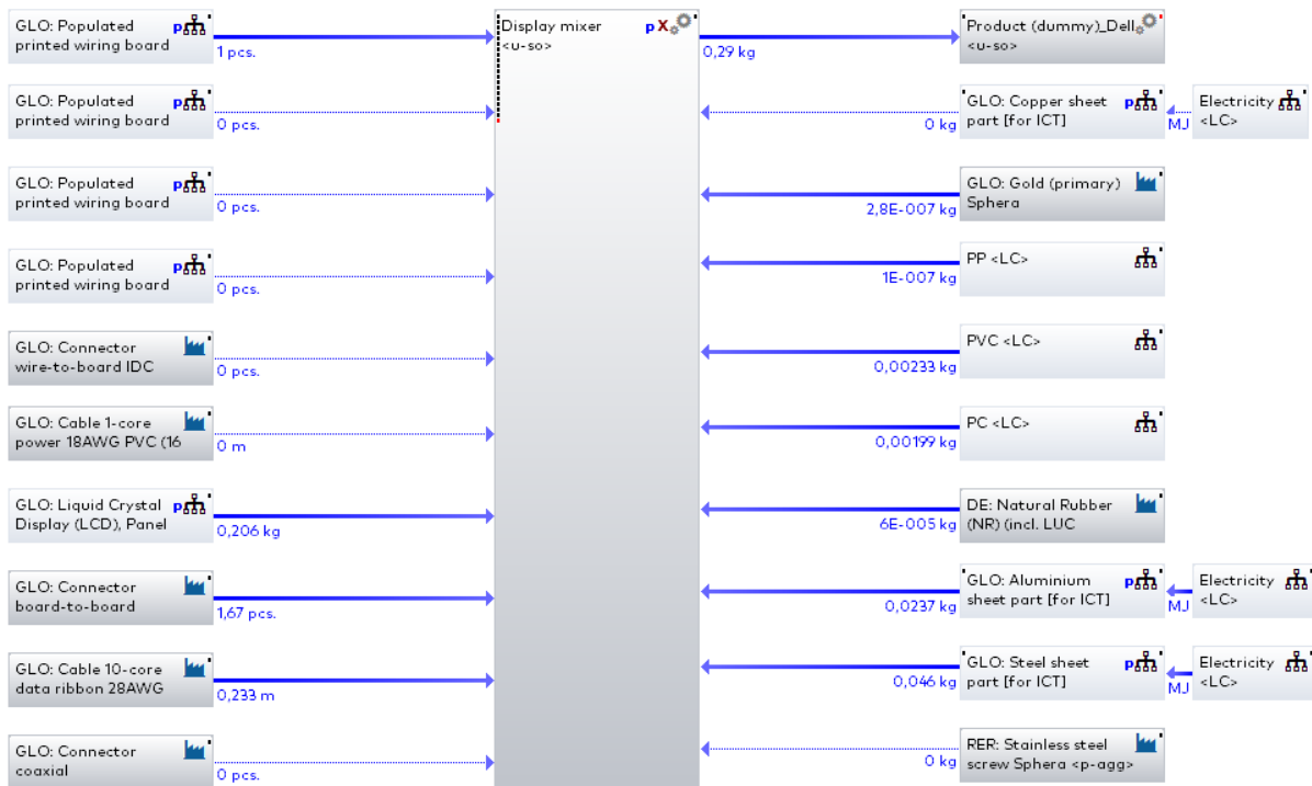
Figure 6-26: Display plan model structure (same for all four notebook types)
