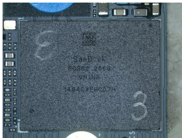
Figure 2-6: Close-up picture of SSD IC
