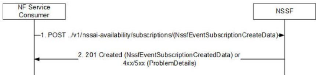
Figure 46. Subscribe service test call flow
