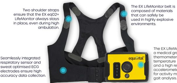
The EX LifeMonitor includes a medical grade infrared thermometer that measures temperature every 15 secs and a high resolution tri-axis accelerometer providing data for activity monitoring and
