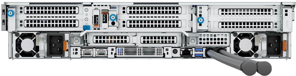
Figure 8. Rear view of the system with optional liquid cooling
