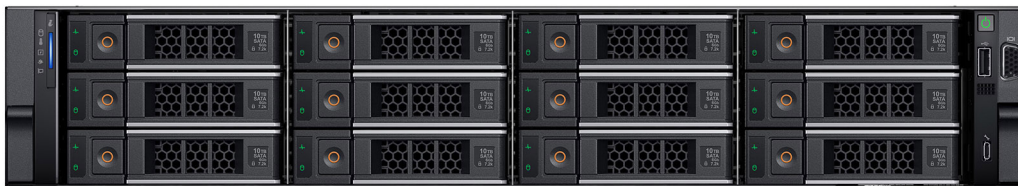
Figure 4. Front view of 12 x 3.5-inch drive system
