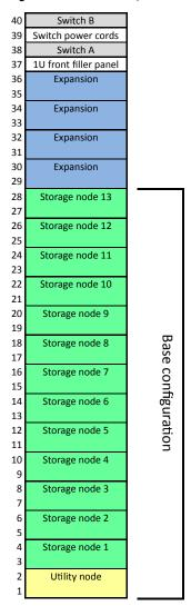
Previous component replacement might have changed the arrangement of nodes in your rack. Since a spare can replace any defective storage node, and because a replacement node can become the new spare, the location of any specific storage node can vary over time.
