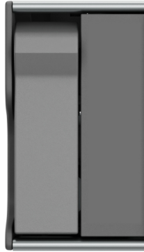
Figure 5. Left Control Panel (LCP)- Secondary panel - blank module
