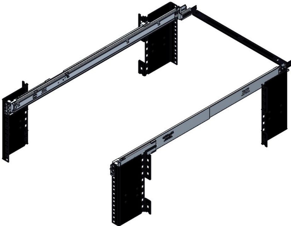
Figure 29. Sliding rails with optional SRB
