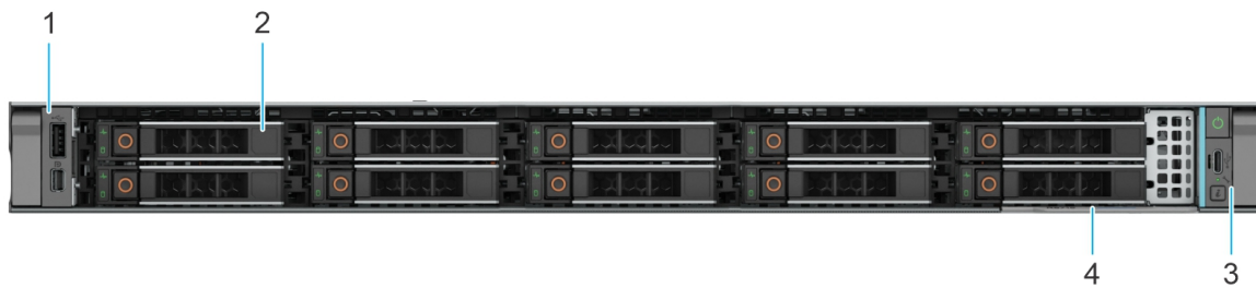
Figure 4. Front view of 10 x 2.5 inch -drive system with rear I/O
