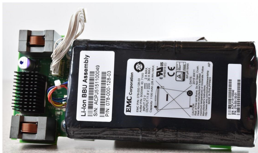
Figure 6. Battery Backup Unit (380/F)
