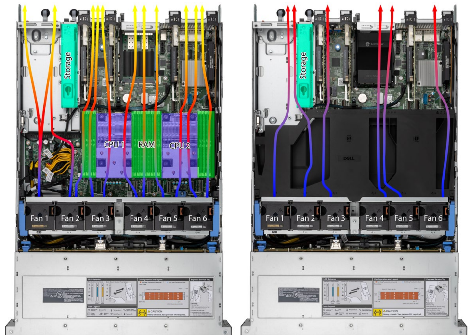
Figure 2: The motherboard layout of the Dell PowerEdge HS5620 we tested, showing the bottom thermal layer (left) and the top thermal layer (right) that the shroud divides. We added component labels and arrows that show airflow direction from the fans, with colder air indicated by blues and purples, and hotter air indicated by reds, oranges, and yellows. Source: Principled Technologies.
