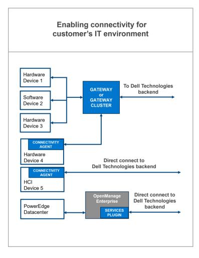
The secure connect **gateway option** allows you to connect your Dell systems to the gateway to communicate back to Dell Technologies Services. This simplifies your firewall / networking set up so that the gateway is the only thing connecting outbound over the internet.
