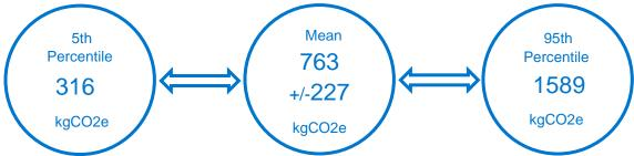
Carbon footprint calculations have a wide range based on a variety of factors including how the device is configured, where it was manufactured and more. Dell Technologies reports the 5th and 95th percentile of the carbon footprint estimate to reflect that uncertainty. For this product, that estimate has a mean of 763 kg of CO2e and standard deviation of 227 kg of CO2e.
